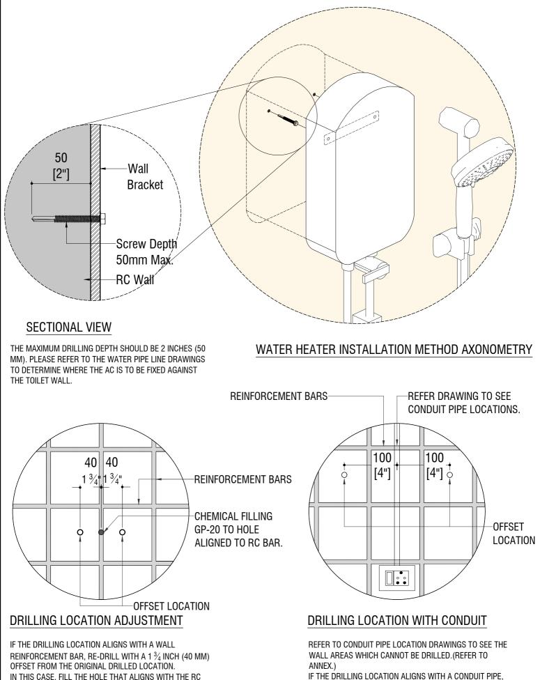
IN THIS CASE, FILL THE HOLE THAT ALIGNS WITH THE RC BAR USING GP-20 HIGH STRENGTH NON-SHRINK GROUT.
